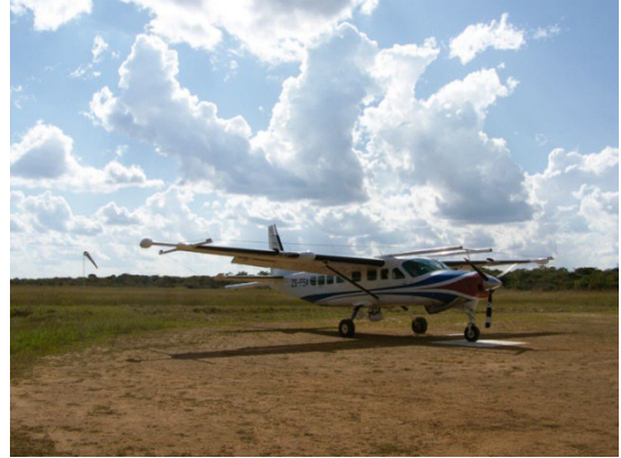
Figure 1. TEMPEST® System installed on a Cessna 208 Grand Caravan.
