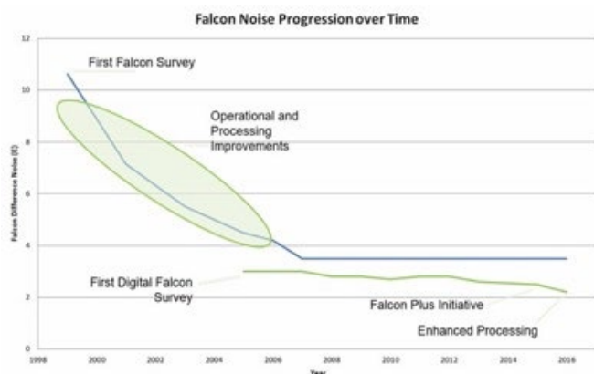
Figure 2: Improvement of noise levels with time obtained with equipment development and enhanced processing techniques. © Xcalibur Smart Mapping
